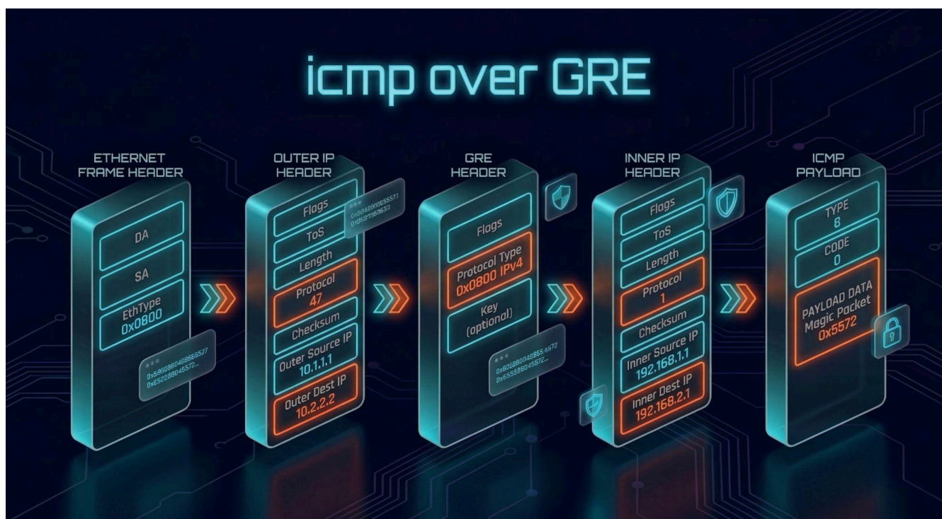
Figure 10: ICMP over GRE tunnel
