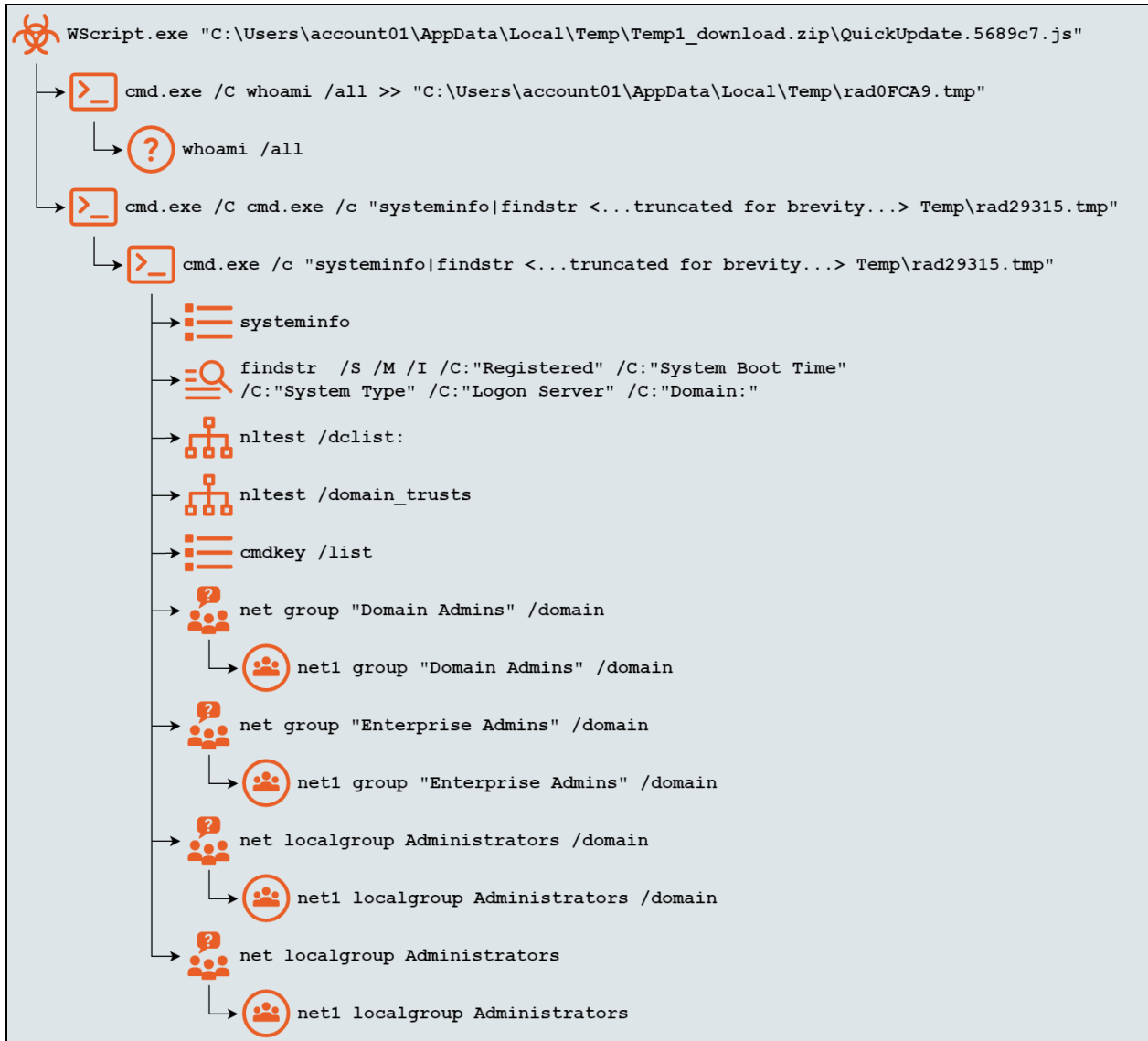
Figure 5 - Process Tree of Initial Discovery Commands Spawned By QuickUpdate.5689c7.js
